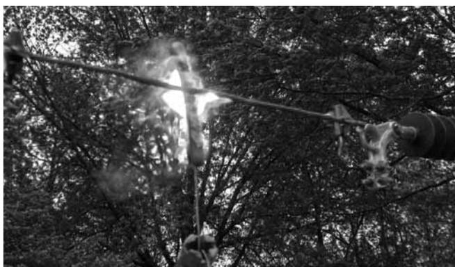
*Hot dogs are used in a simulation to show the effects from when a human person comes in contact with a high voltage power line. The line that the hot dogs are touching is 7,200 Volts.*
