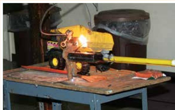
▲ This part of the demonstration uses a Tonka Truck to illustrate the hazards of operating large equipment around power lines and the dangers associated to those trying to rescue someone from a vehicle in contact with energized lines.
